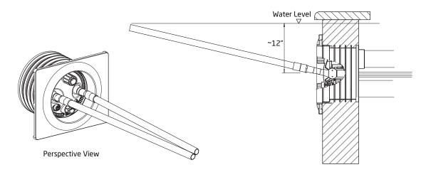
Figure 4 - BaduJet Nozzle Adjustment
