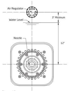
Figure 13 Installation in Concrete or Gunite Pools
