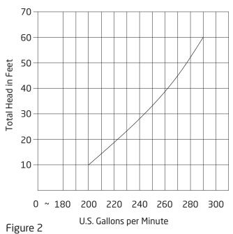
BaduStream II Head Loss Curve (Single Jet Housing)
