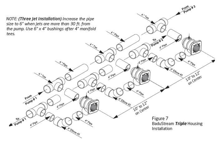
IMPORTANT NOTE: **CHECK VALVES <u>MUST BE</u>** used on the discharge side of each pump. Minimum 4" pipe between pump and BaduStream plumbing manifold.
