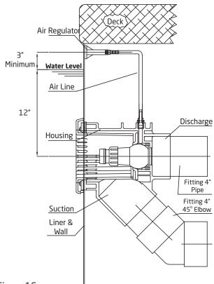
Figure 16 <sup>II</sup> BaduStream in Liner or Fiberglass Pool.
