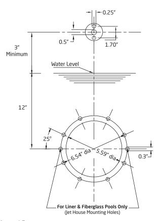
Figure 15 Cutout Pool Wall for BaduStream housing.
