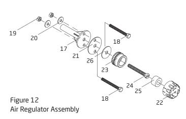
D. Install the hose ring (part #25) and snap the top part of the air regulator (part #22) into place. See Figure 12 for air regulator assembly.
